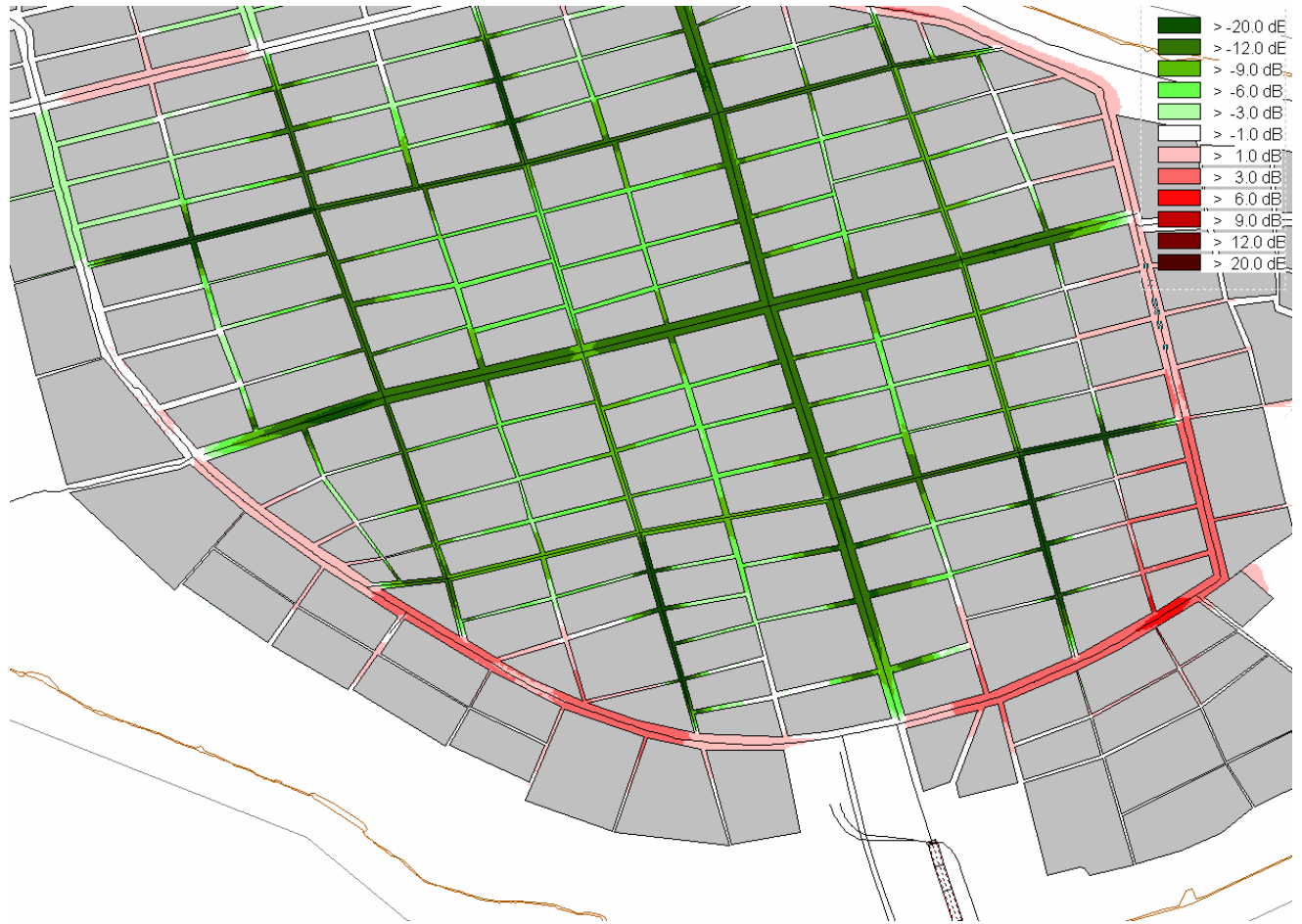
Fig. 8. Difference map for the entire Quiet Zone for Scenario #2. Application of closing gates for noisy vehicles.
