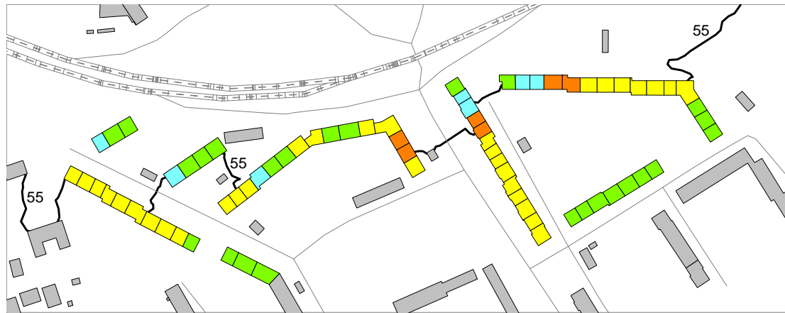
Figure 4: Hot-spot analysis after implementing substantial window measures to all apartments with a façade level above 65 dB(A).
