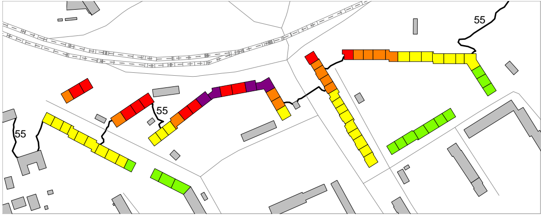
Figure 3: An analysis is made of the present situation for comparison with the results from the different measures. The black line represents the calculated 55 dB(A)-line.
