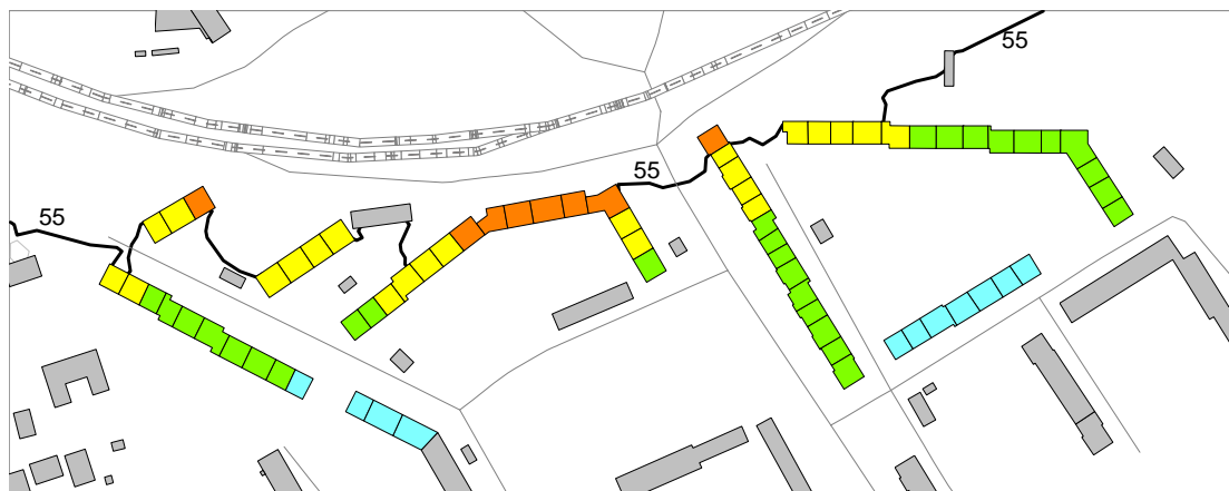
Figure 6: The results of the sound reducing asphalt shows clearly in the hot-spot analysis.
