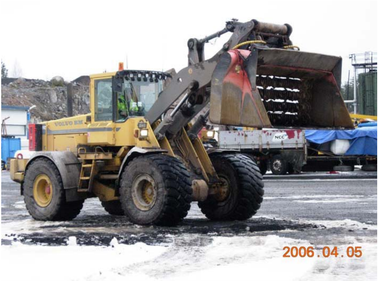
Figure 2. Shredder (type ALLU) used for disintegrating the impregnated crumb rubber.
