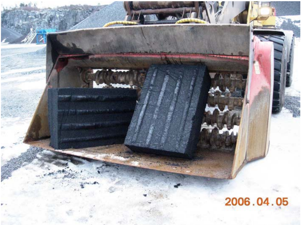
Figure 3. Blocks of impregnated crumb rubber before the disintegration process before feeding the impregnated and pulverized crumb rubber to the plant mixer.
