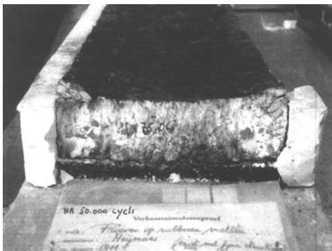
Figure 16. Test plate with SMA-C2 after rutting test.
